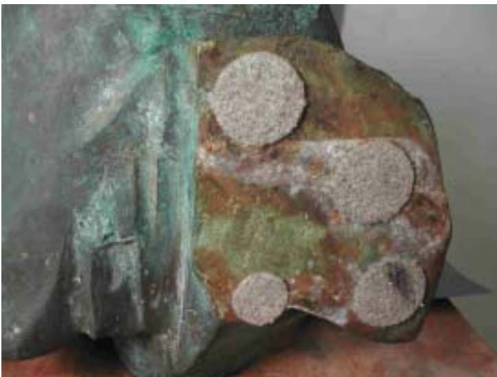
An example of a heavily corroded underside (above left). Original patina has been lost. It was repatinated and coated with a protective lacquer (above right).
