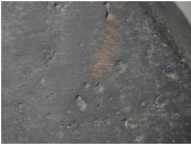
Scratches and abrasions of the surface of a bronze sculpture due to handling.
