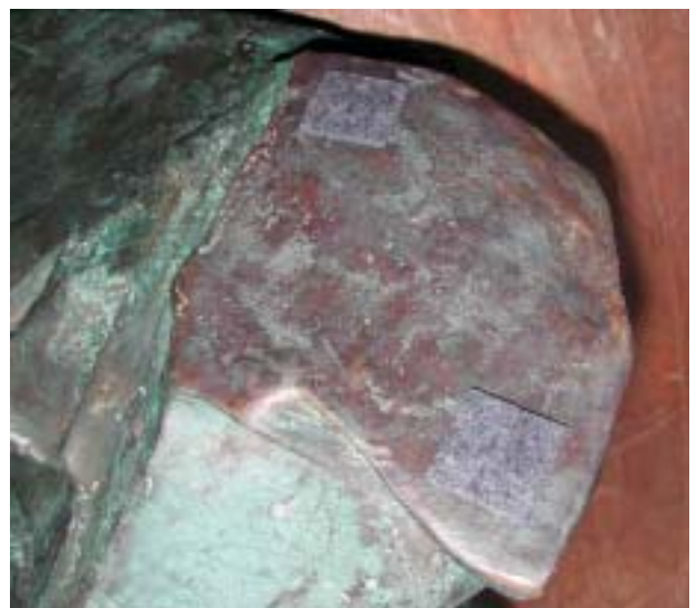
An example of a heavily corroded underside (above left). Original patina has been lost. It was repatinated and coated with a protective lacquer (above right).
