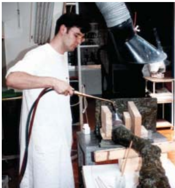
Alberto Giacometti's La jambe being handsoldered due to a massive fracture in the ankle.
