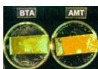
Figure 5: After corrosion at 95% RH. (41K)
